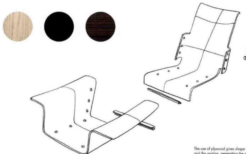
The use of plywood gives shape to the structure and the seating, generating the armrests that support the position of the body, and offer a multitude of possible uses due to their generous dimensions.
